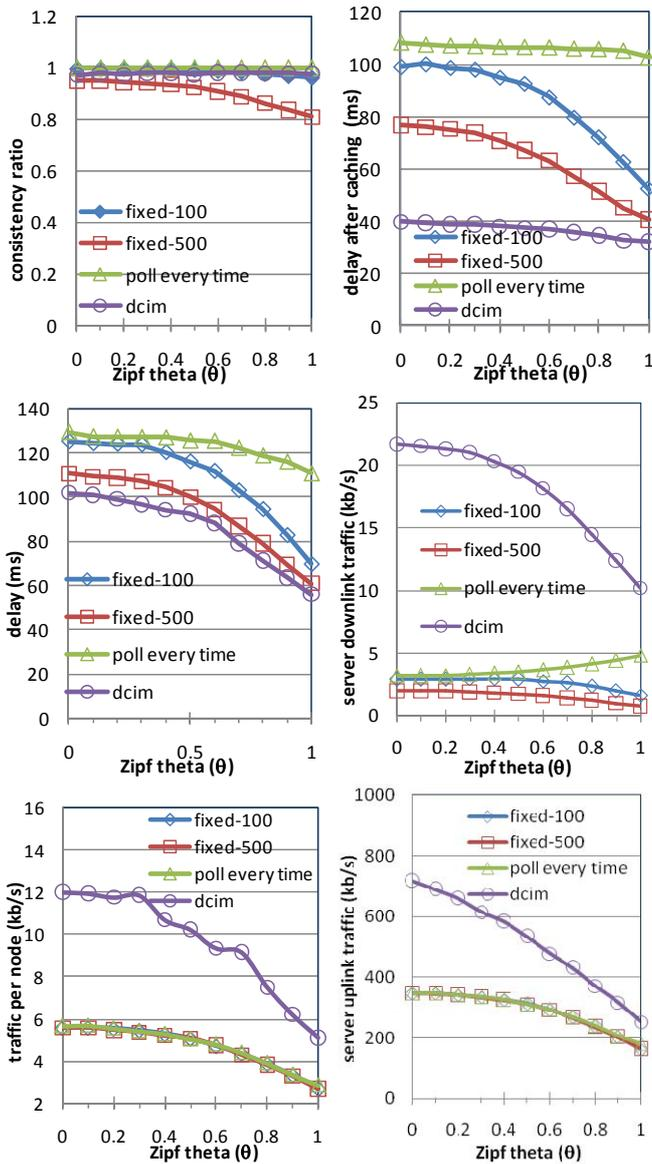
Fig. 9. Performance measures versus the zipf parameter
