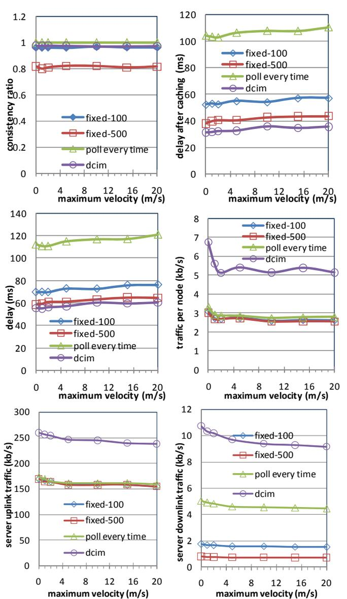
Fig. 10. Performance measures versus the node maximum velocity
