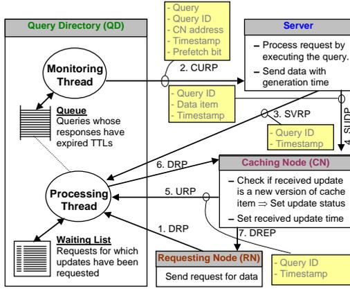
Fig. 2. Interactions between nodes in a DCIM system
